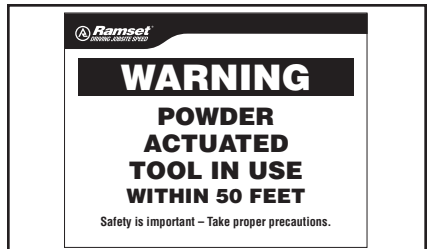
ALWAYS POST WARNING SIGNS
